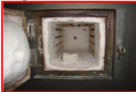
Fig. 4e: Pre Heating of the Cast
